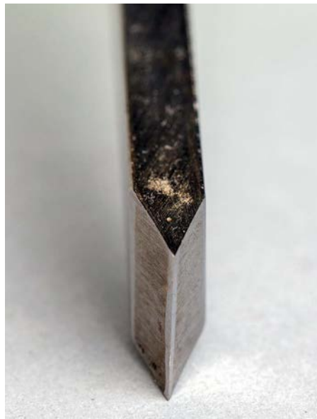
I use a bench grinder for a hollow grind on my skews letting me touch them up with a diamond hone
