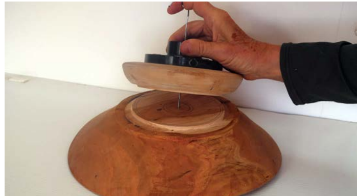
An example of a glue block union being positioned on an already rough-turned bowl. This method could be used to mount a new blank of wood ready to be turned
