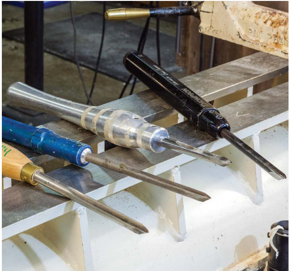
Four modern spindle gouges made from HSS bar stock. (L–R) A standard Hamlet spindle gouge; Sorby, Henry Taylor, Crown Handtools and many more companies make very similar gouges; a Jerry Glaser detail gouge which has a shallower flute and was his innovation; a Carter and Son detail gouge made from M42 HSS; a Thomson Tool made from powdered steel
