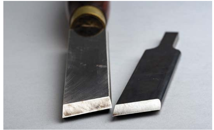
You can buy skews handled or unhandled. Opting for the larger sizes provides a larger sweet spot
