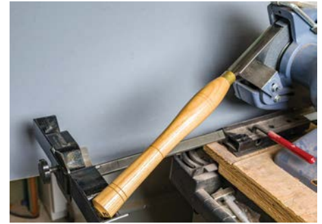
The skew jig attachment to the Wolverine makes sharpening quick and easy
