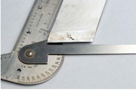
All of my skews fall in the 70° range although I eyeball them when grinding rather than measure
