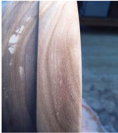
Cabinet scrapers can be used to great effect, but if you are unsure about freehand scraping, use a conventional scraper placed on the rest and presented in shear cutting mode or use a dedicated angled shear scraper to remove minor imperfections
