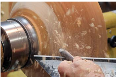
A pull cut is an option to remove bulk, but is not as good at refining a surface as a push cut
