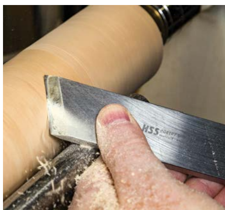
The skew excels at the planing cut. Stay in the sweet spot with a sharp tool and light touch
