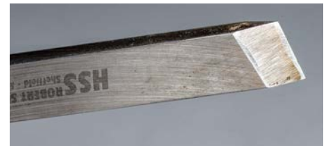
Grind surfaces aren't parallel or the cutting edge isn't dead centre? A sharp cutting edge works
