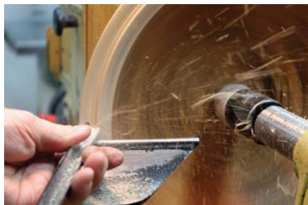
The push cut is the go-to cut for optimum shaping and refinement
