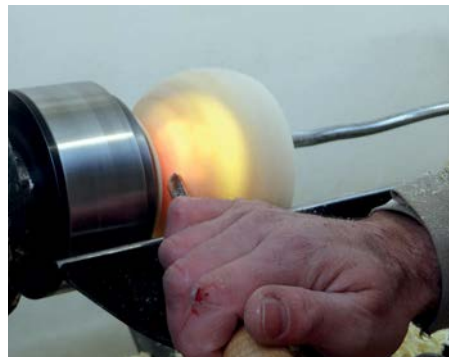
Using the light inside the bowl to finish the base and part off
