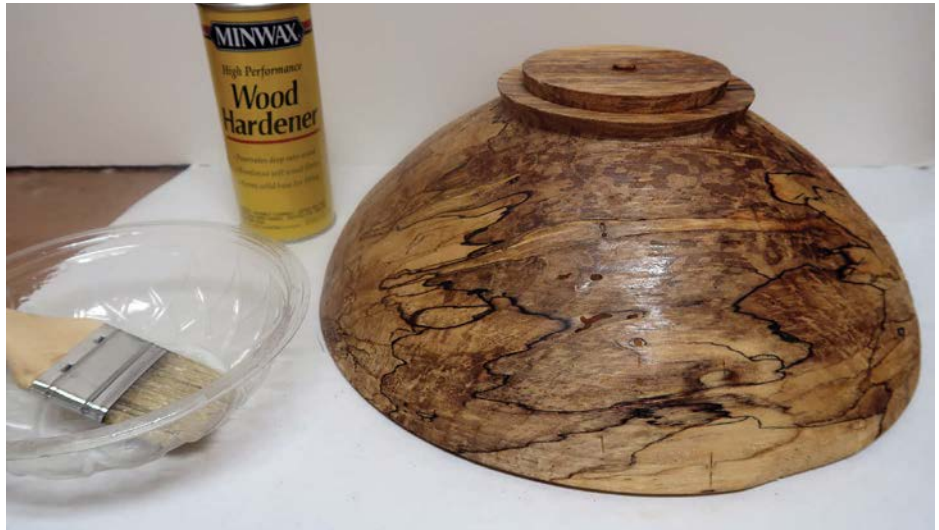
This bowl has had complete saturation of wood hardener all over
