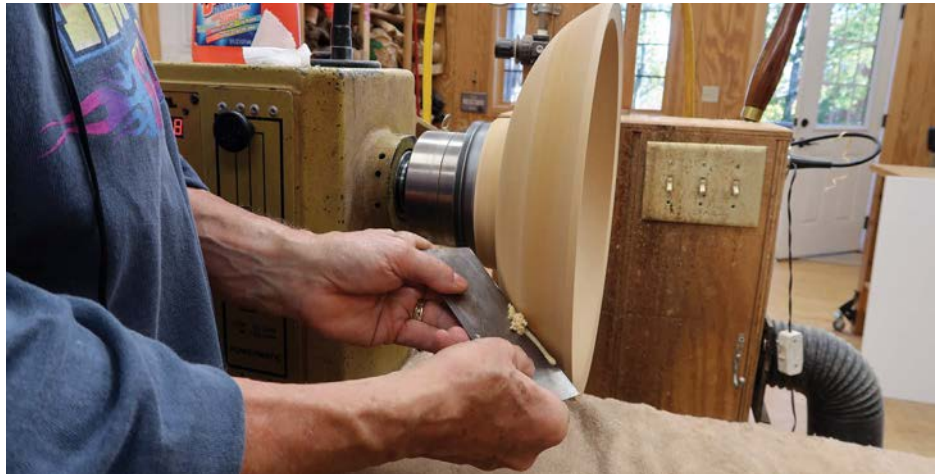
Cabinet scrapers can be used to great effect, but if you are unsure about freehand scraping, use a conventional scraper placed on the rest and presented in shear cutting mode or use a dedicated angled shear scraper to remove minor imperfections
