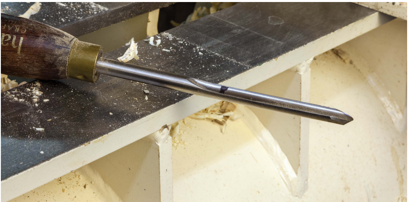
A combination gouge has a flute milled deeper in the round bar and cannot be ground to as long an angle. Great for cleanup cuts in faceplate work, it does not turn spindles as well as a true spindle or detail gouge
