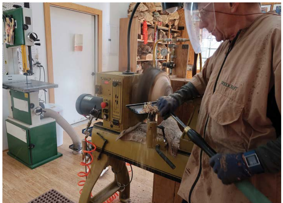
Always stand out of the line of fire – the potential exit point – of work while you turn
