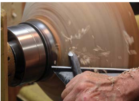
A shear cut is a cut that may – or may not – improve upon a push cut
