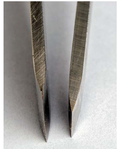
You may wish to try a convex grind. It has some forgiving qualities for the newcomer
