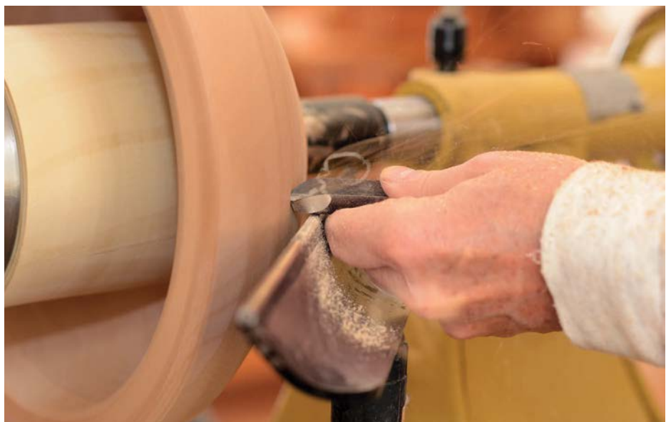
Initial mounting of the hardened rough-shapes bowl between centres in order to refine the outside shape
